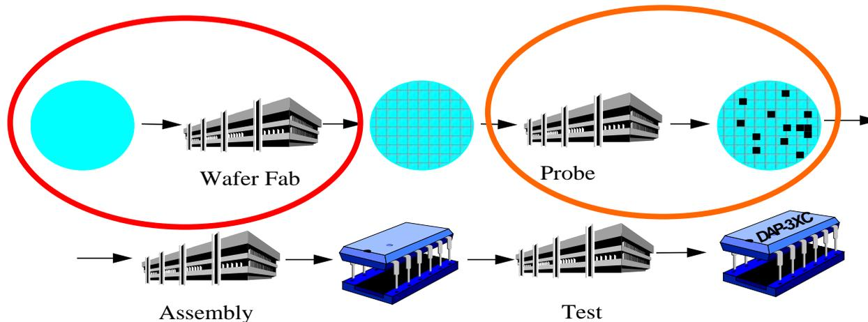
3. Probed wafers are sent to **Assembly** where good dies are put into a package.
